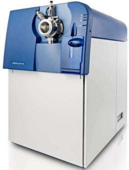
LC-MS/MS high resolution API 5600 QToF
