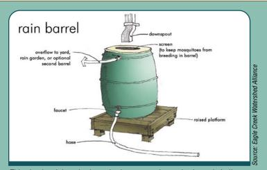
This simple rainbarrel schematic shows a gravity garden hose drain line.
