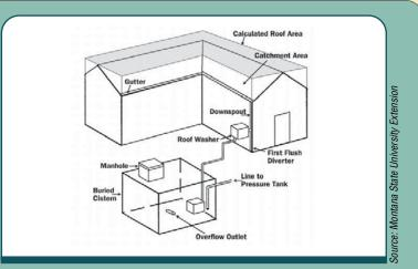
This variation of a cistern system uses an underground tank and pumped supply line.
