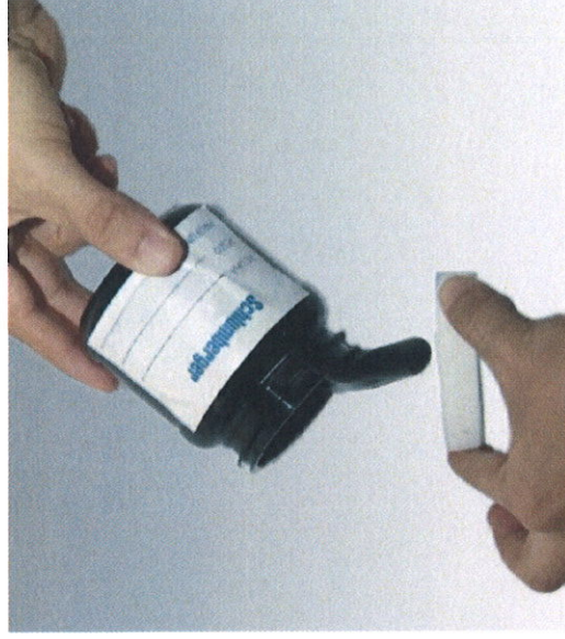
The Saturn 3D radial probe collected an uncontaminated sample of 7.5-API oil from an unconsolidated sandstone reservoir without sanding or seal failure.
