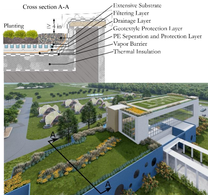
Figure 17. Components of proposed green roof for the MAST building
