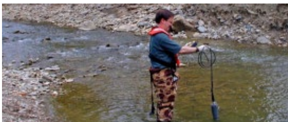
Figure 8. Measuring temperature in the field. Credit: Photo courtesy of USGS
