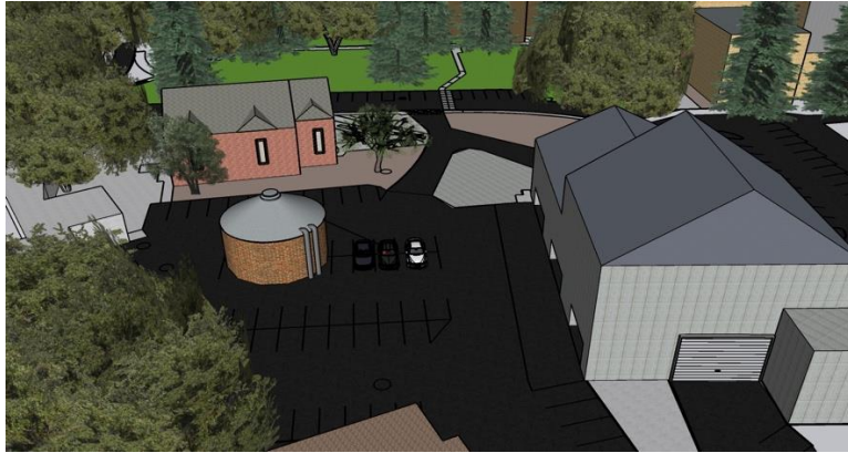
Figure 4. Above ground cistern that would store treated stormwater runoff. The brick exterior matches the UP building aesthetic.
