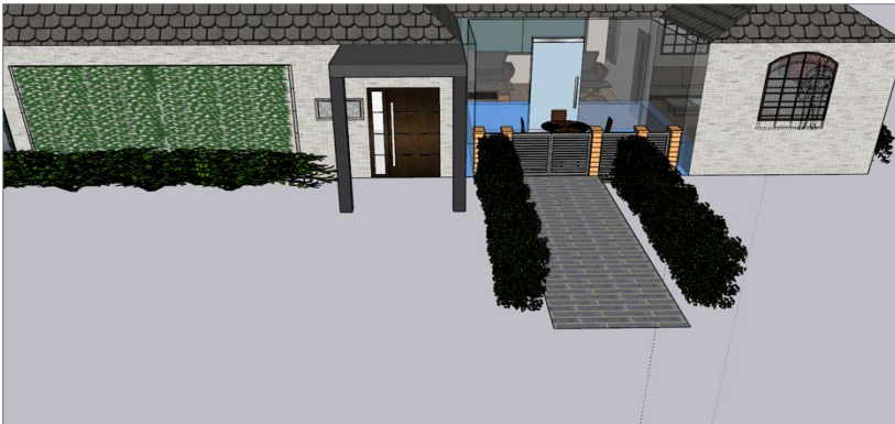
Figure 9. The exterior of the front side of the Mental Health Haven is located on the Northeast side of the bluff with a small-scale living wall, permeable pathway, and small bioretention planters.
