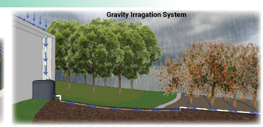
The 5,000 gal cistern, located 10ft above the persimmon orchard, harvests stormwater from the roof of the garage and takes advantage of the gravity to save more than 565 KJ energy for each irrigation/ cistern.
