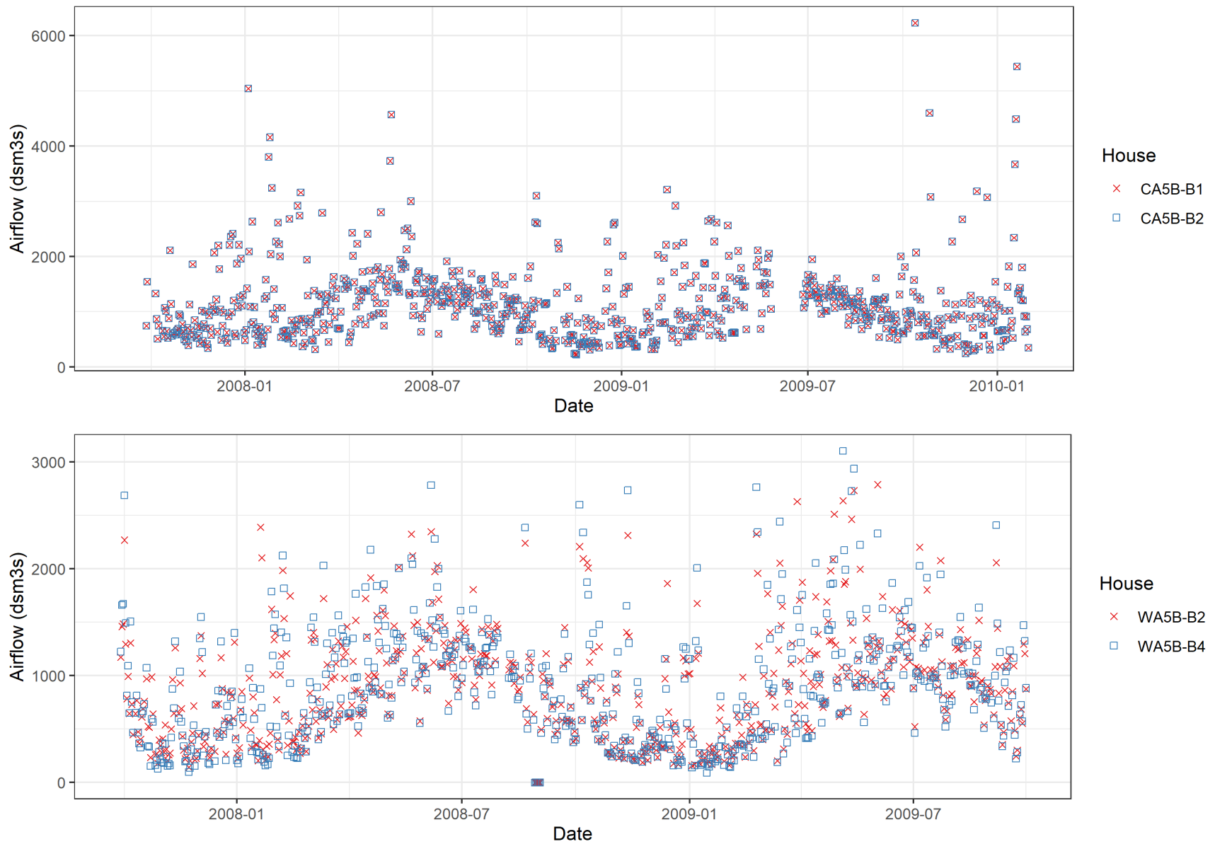
Figure E-39. Trends in airflow rate at naturally ventilated barns, by site, during the NAEMS monitoring period.
