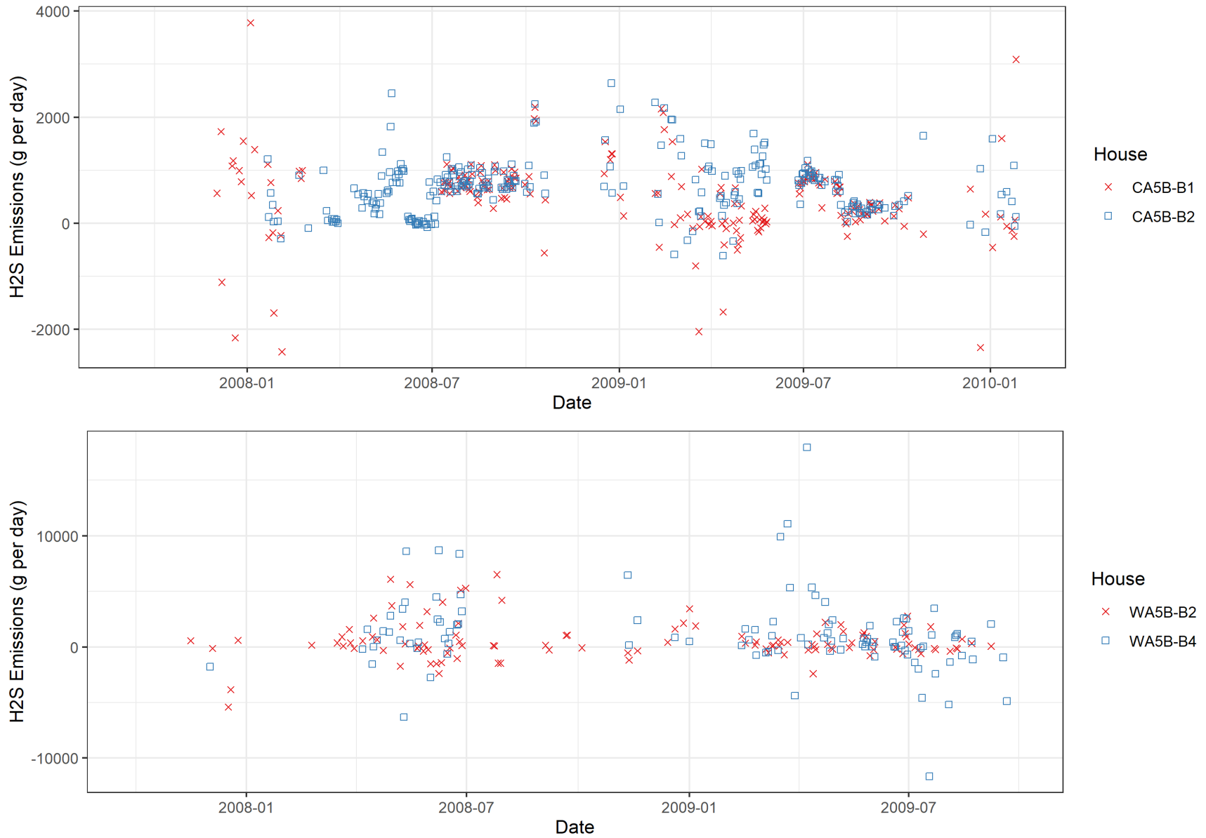
Figure E-30. Trends in H 2 S emissions at naturally ventilated barns, by site, during the NAEMS monitoring period.
