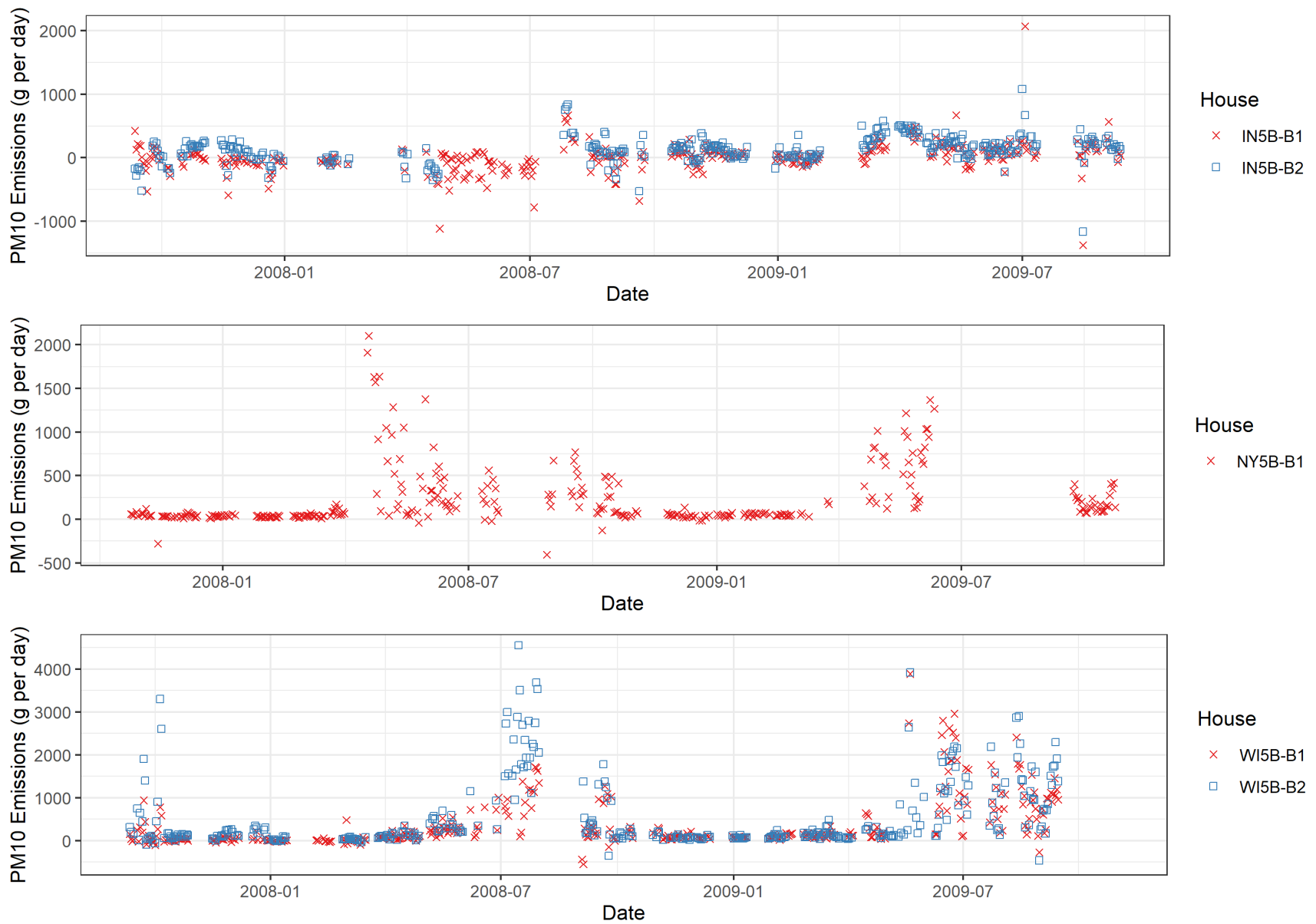
Figure E-3. Trends in PM 10 emissions at mechanically ventilated barns, by site, during the NAEMS monitoring period.
