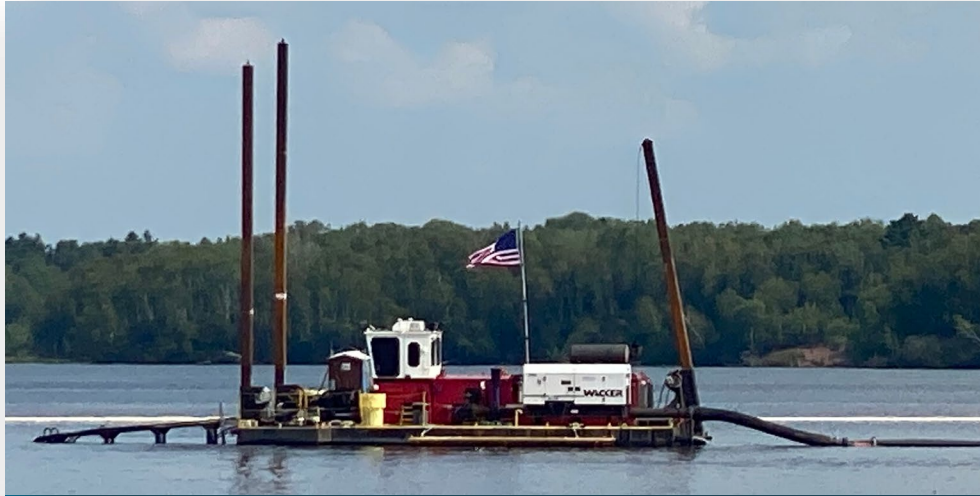
Hydraulic dredge sits on a barge in the Wire Mill Delta.
