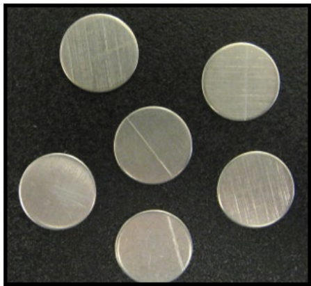
Fig. 2: Examples of typical unacceptable carriers.
