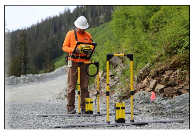
Figure 5: GPR pulseEKKO PRO System, with 50-MHz Antennae Frequency
