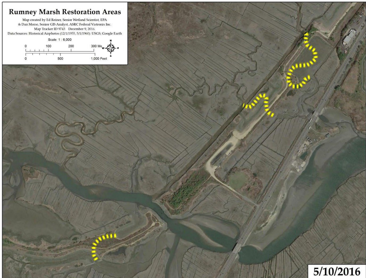
Figure 33. Aerial photo taken May 10, 2016, highlighting the locations of former channels which were filled along the abandoned I-95 embankment in Revere and Saugus, Massachusetts.
