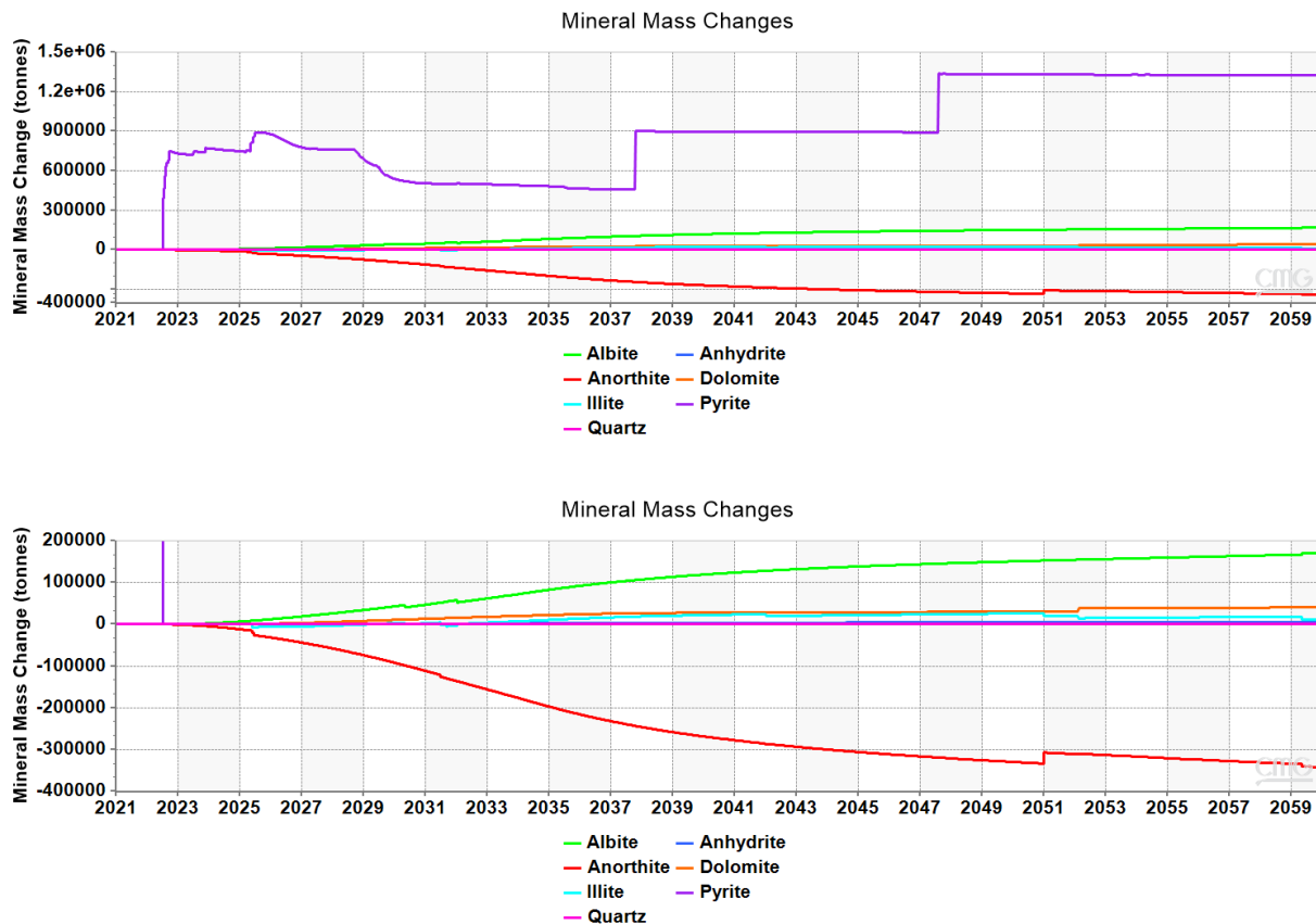
Figure 2-25. Dissolution and precipitation quantities of reservoir minerals because of \text{CO}_2 injection. Dissolution of anorthite with precipitation of pyrite, albite, and dolomite was observed. Upper figure shows all the minerals; the lower figure is rescaled for better view of the minerals mass change except pyrite.
