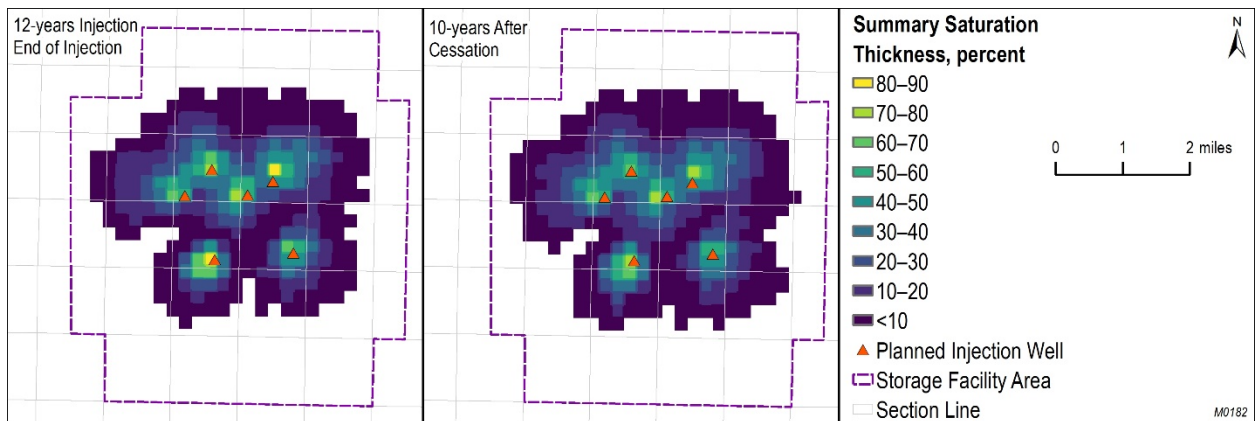
Figure 5-6. Simulated extent of the CO 2 plume at the cessation of injection and the postinjection stabilized plume.
