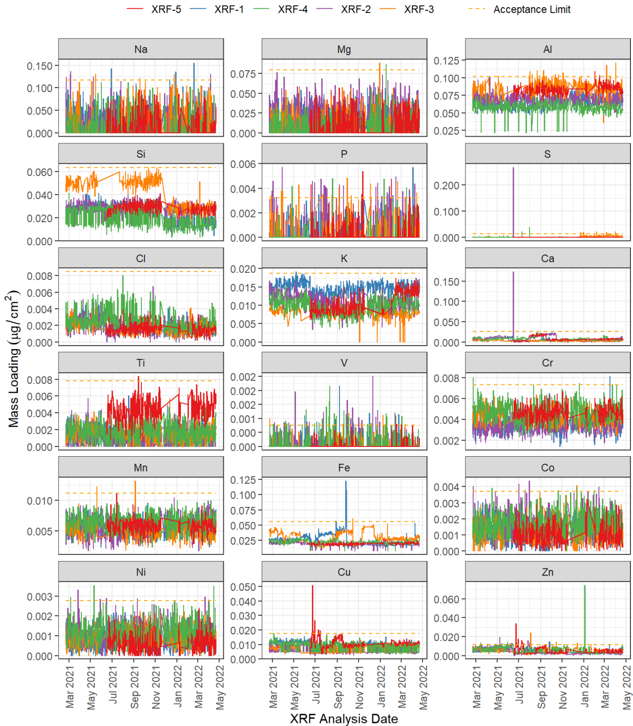
Figure 4.2-1: Analysis results from daily PTFE blanks for the analysis period 2/19/2021 through 4/22/2022 (see Table 4.2-1 for corresponding sampling dates). Elements Na through Zn shown.
