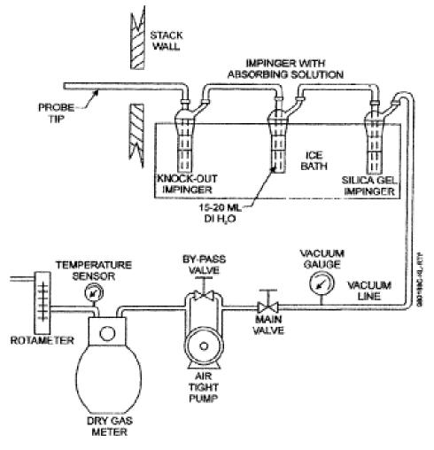
Figure 323-1. Chilled Impinger Train Sampling System
