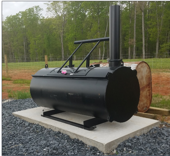
Figure 2. An animal waste/mortality facility installed along Turpin Creek.
