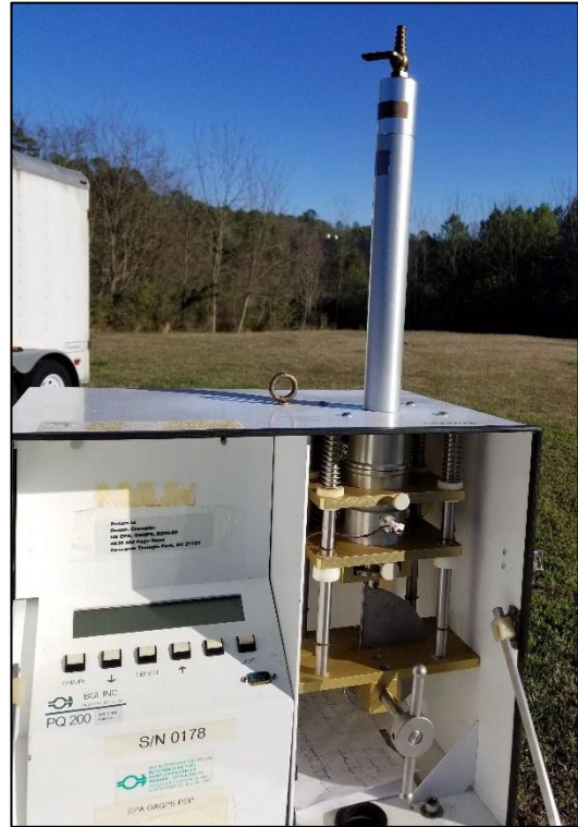
Figure 6-3a. Photo of flow rate adapter for the PM 2.5 -PEP sampler
