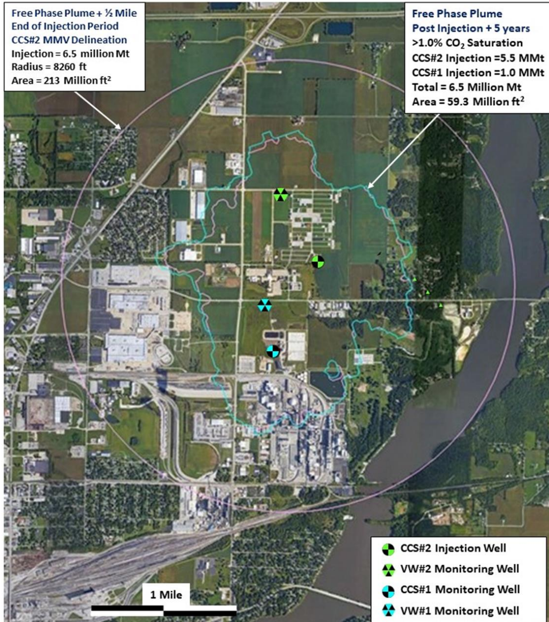
Figure 2. Active Monitoring Area (AMA) is defined by plume outline (pink) at the end of the injection period plus ½ mile buffer (pink circle). The plume outline at the end of the injection period plus 5 years is shown by the blue outline.
