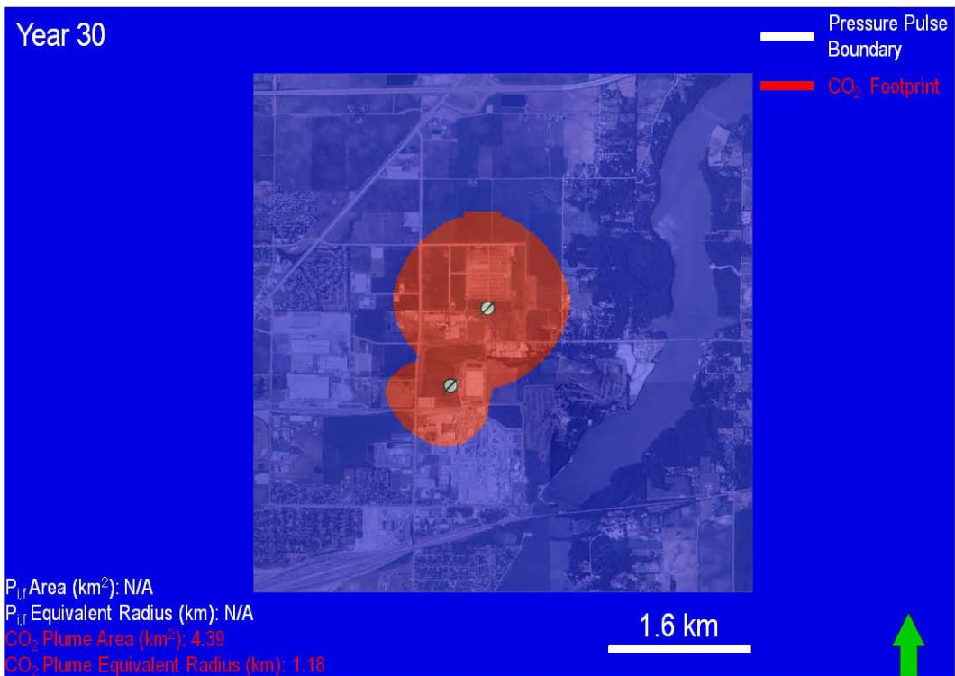
Figure 5-20: Map-view of pressure front ( P_{i,f} ) and CO 2 plume footprints after simulated Year 30.
