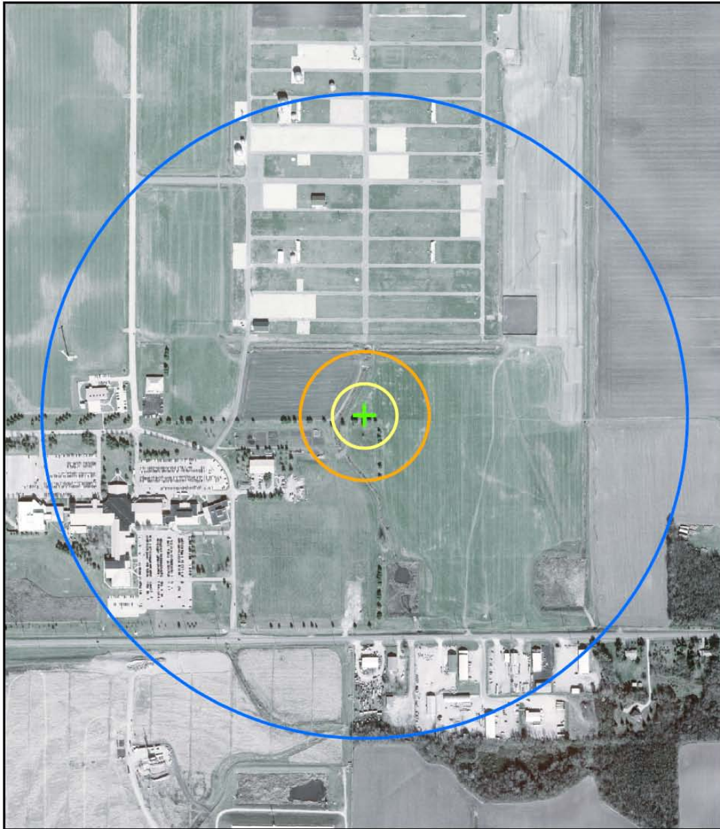
Figure F-1. IL-ICCS Injection Site Showing Groundwater Compliance Well Areas. Two wells will be within 200 feet of the injection site, one within 400 feet, and one within 2,000 feet.
