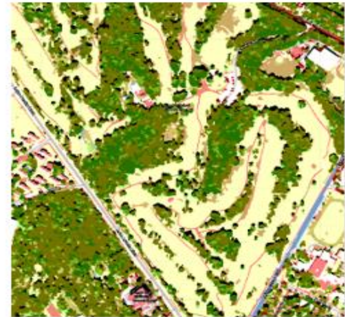
Segmentation (object-based) and machine learning classified cover: tree (green shades), grass (yellow), bare soil (brown), built (grey, red, white)
