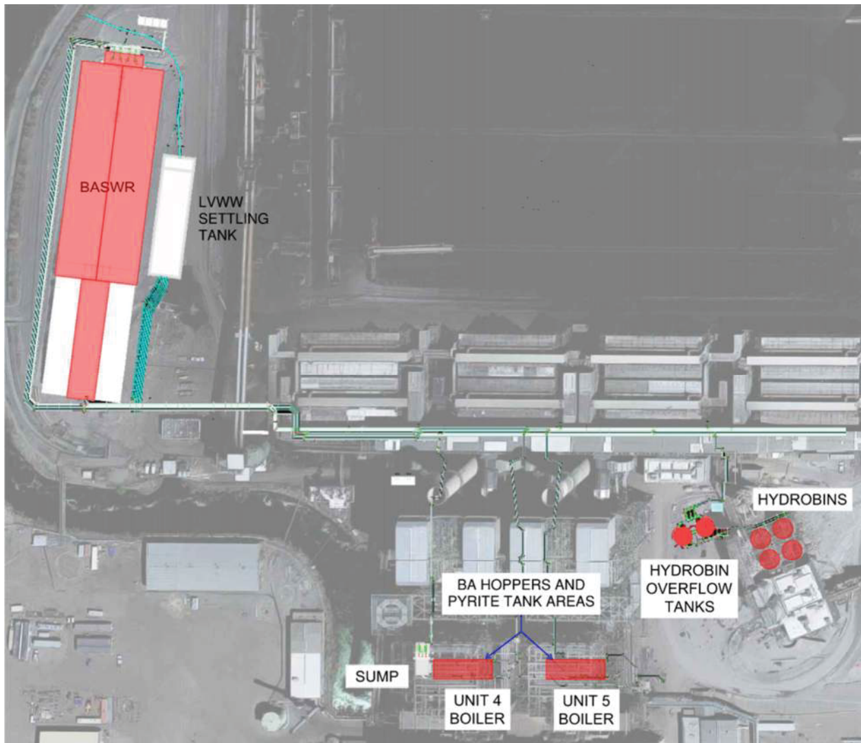
Figure 2-1: Site Plan Showing Major System Components
