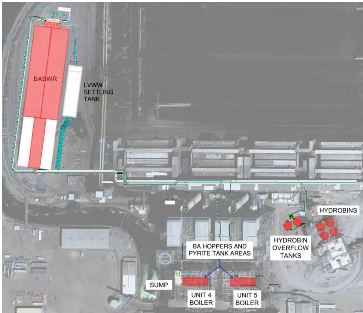
Figure 2-1: Site Plan Showing Major System Components
