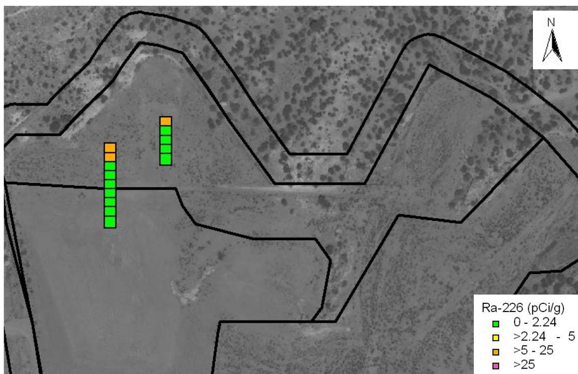
Plate 4.3-8 CR-1 Ra-226 Soil Concentrations Measured with Deep Drilling Program on Former Industrial Area
