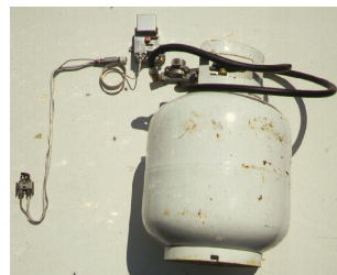
a Pilot light propane heater
