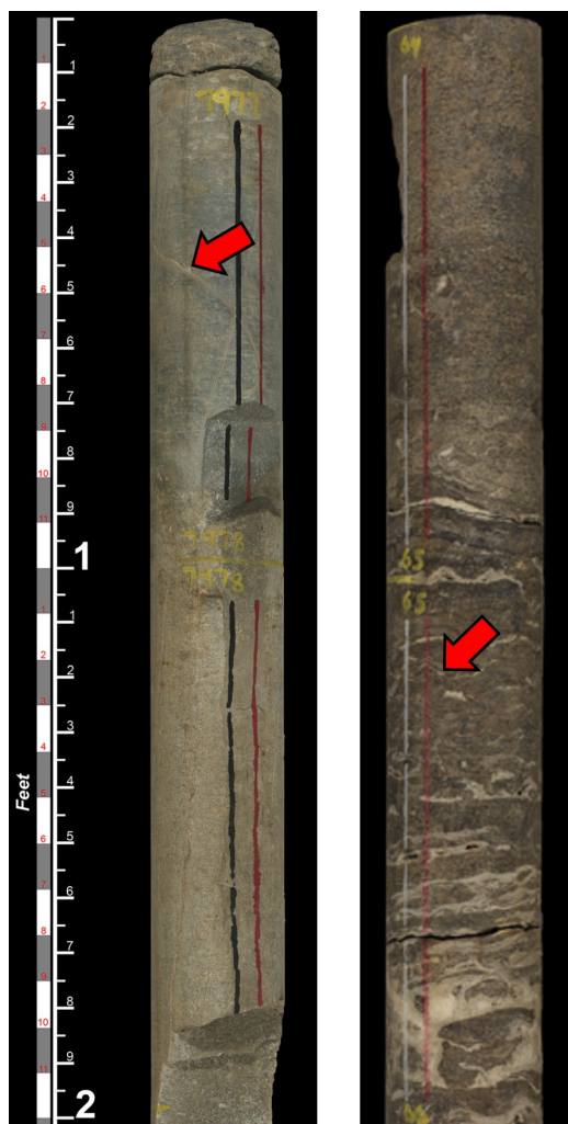
Figure 32: Representative whole core examples of confining (left) and injection (right) zones illustrating natural fractures (generally cemented, red arrows).
