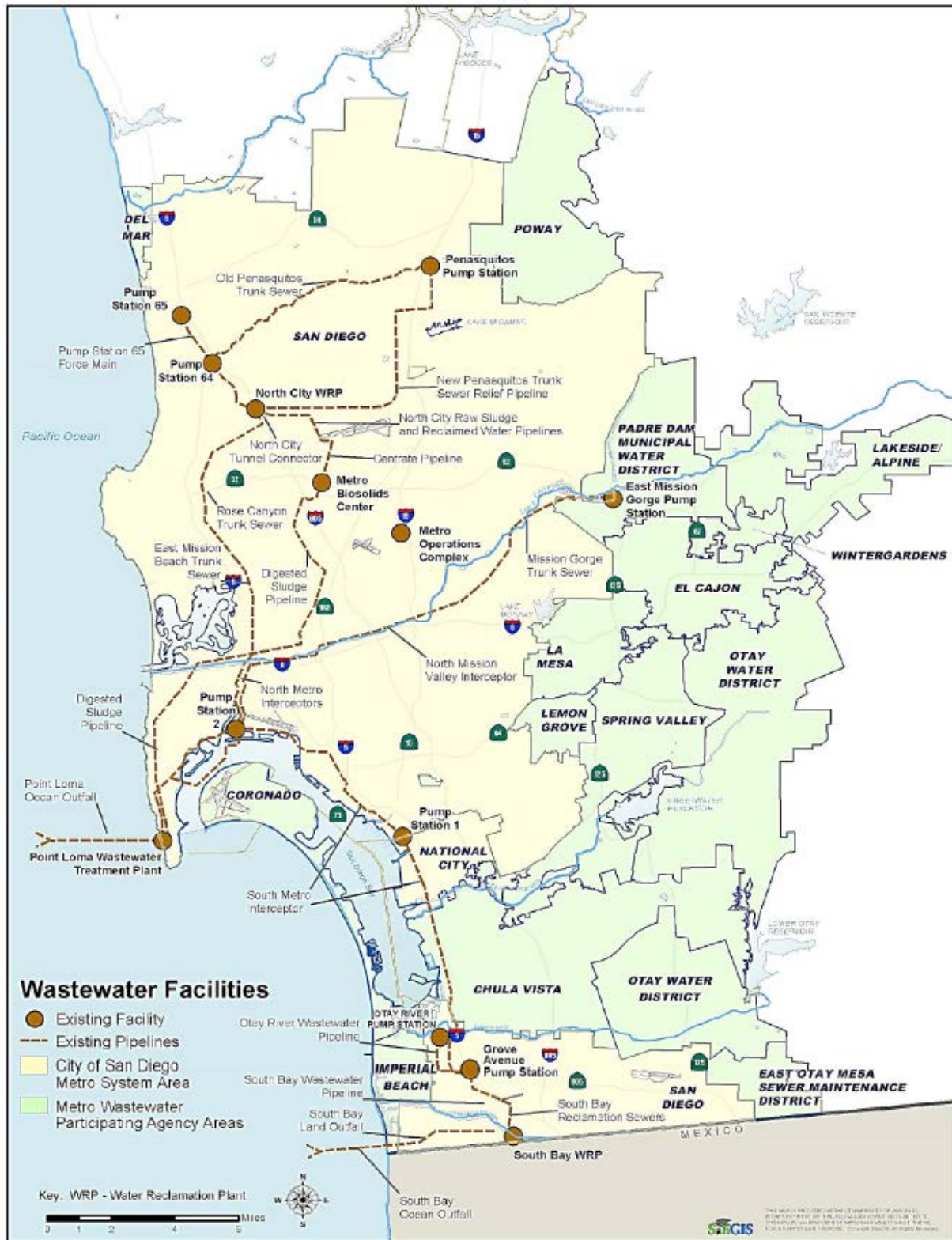
Figure A-1. Map of the San Diego Metropolitan Sewage System service area
