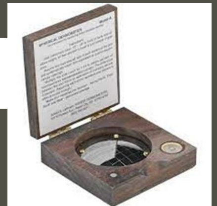
Convex densiometer for estimating canopy cover
