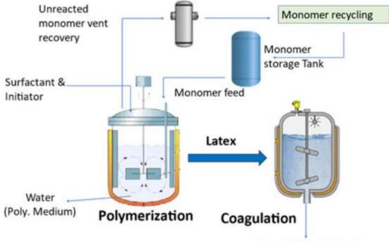
Coagulation drain water (Water + Surfactant) The unreacted monomer, TFE, is collected through a vent recovery process and sent to the monomer recycling unit where - after purification - the monomer is stored in storage tanks for reuse in the polymerization process.
