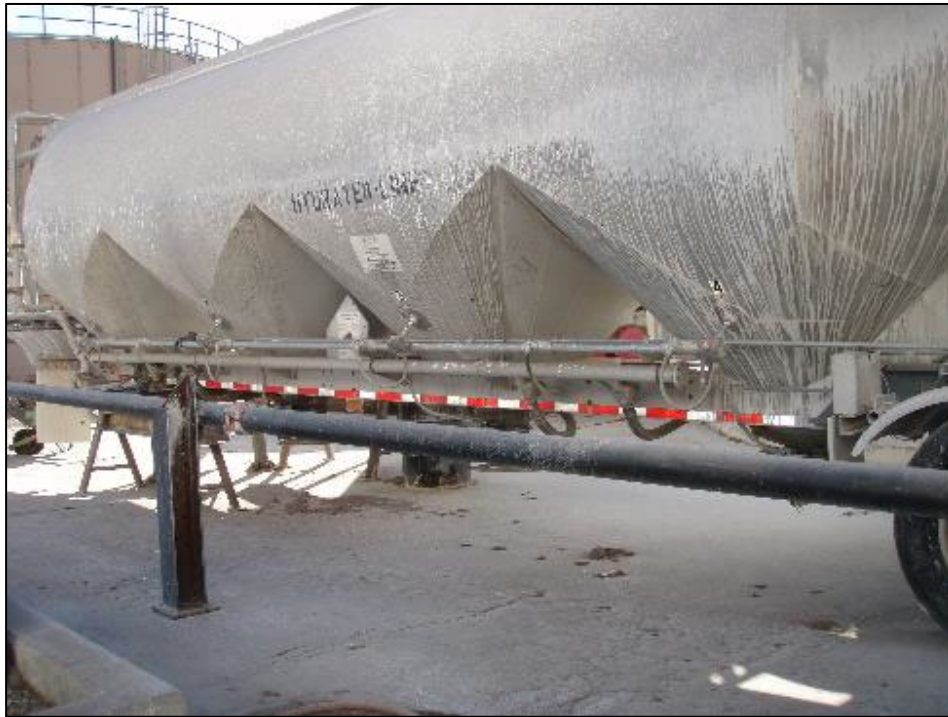
Photograph 4: View of pig trailer storing hydrated lime.
