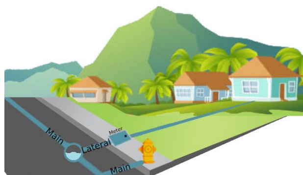
Figure 1. Graphic showing main water line connection to hydrant and residential lateral line.
