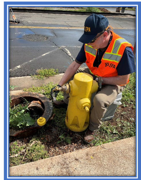
Figure 1. EPA crew member taking a distribution system sample at a fire hydrant.
