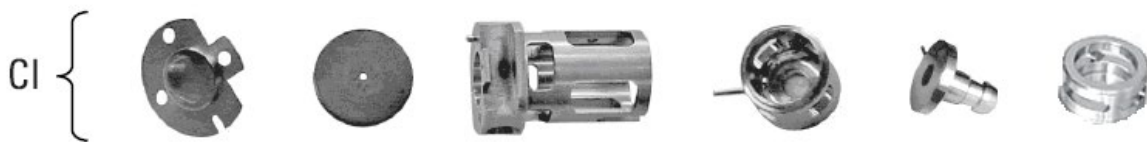
Figure 2. CI ion source parts to clean.
