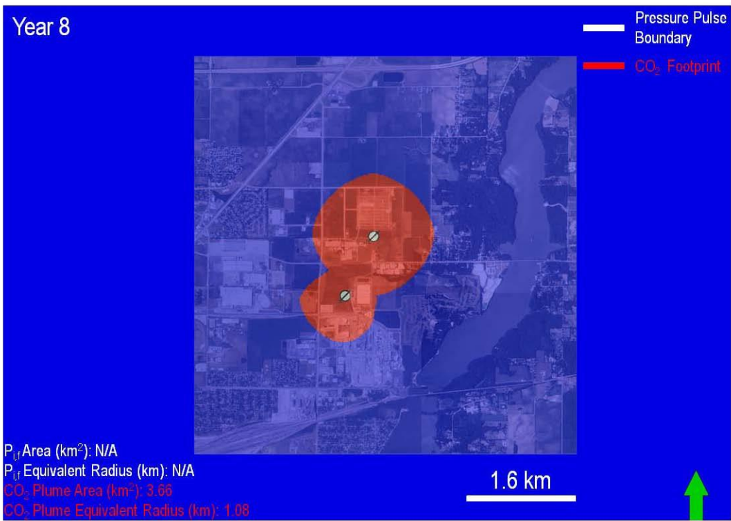
Figure 5-16: Map-view of pressure front ( P_{i,f} ) and CO 2 plume footprints after simulated Year 8.
