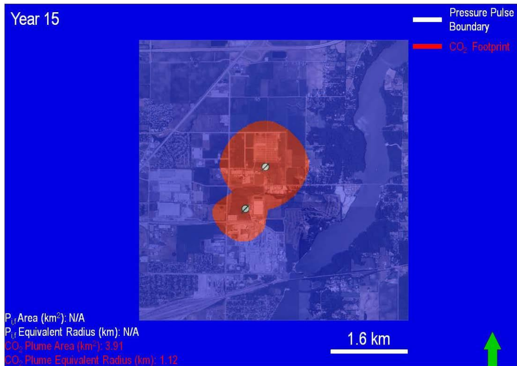
Figure 5-18: Map-view of pressure front ( P_{i,f} ) and CO 2 plume footprints after simulated Year 15.
