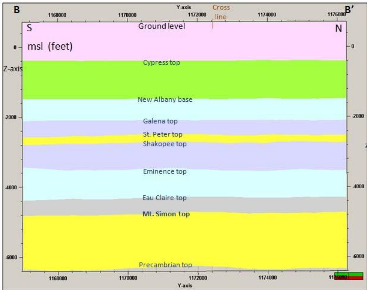
Figure 2-7: Cross section illustrating the geology along south (B) to north (B') direction (location given by Figure 2-5). Source: Smith, Schlumberger Carbon Services, 2011 .
