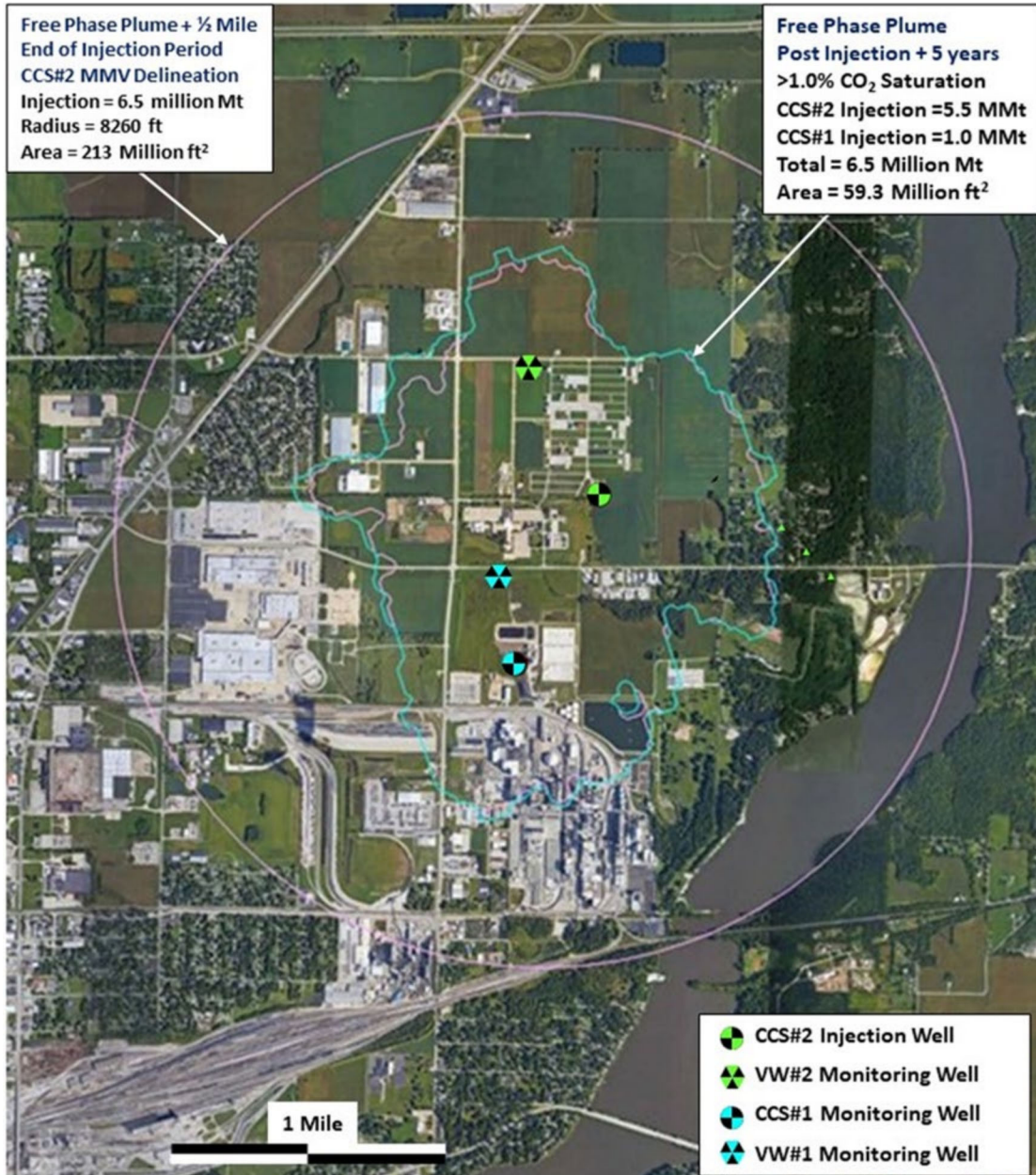
Figure 4. Maximum Monitoring Area (MMA) is defined by the stabilized CO 2 plume (blue) plus a half mile buffer zone (pink circle). The Active Monitoring Area (AMA) is the same as the MMA as described above.
