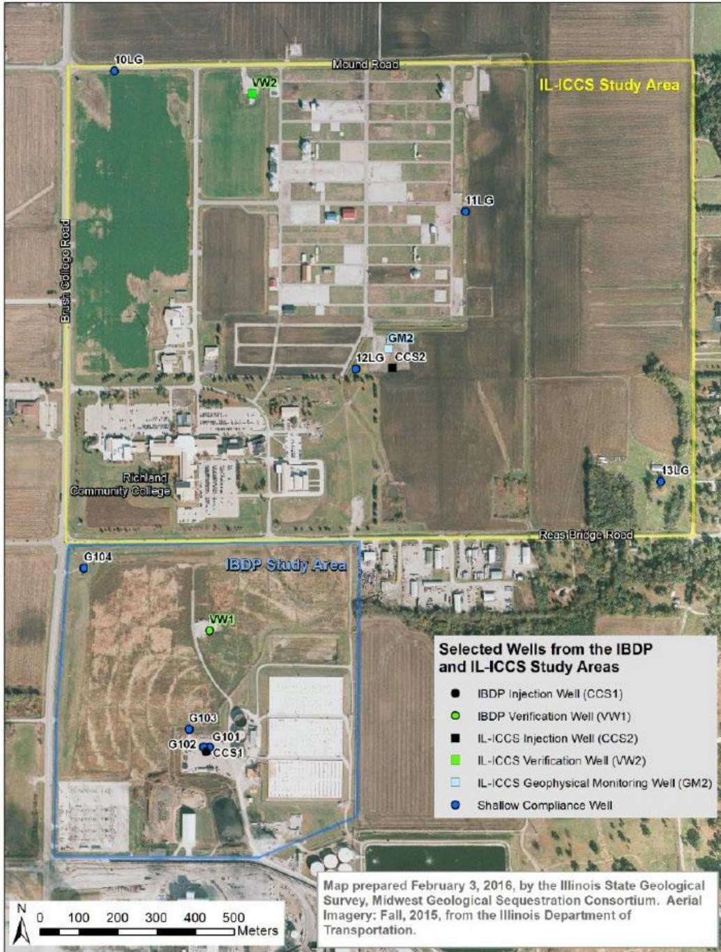
Figure 1. Site map for groundwater compliance locations related to USEPA UIC Permits IL-115-6A-0001 and IL-115-6A-0002.
