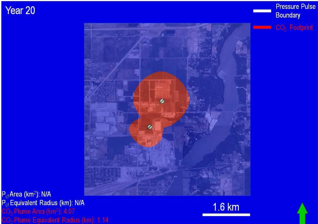
Figure 5-19: Map-view of pressure front ( P_{i,f} ) and CO 2 plume footprints after simulated Year 20.
