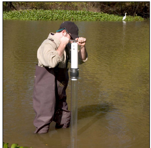
Figure 4. An example of sediment sampling using a core sampler.
