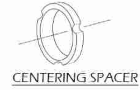
CENTERING SPACER CENTERING SPACERS KEEP THE CARRIER PIPE STRAIGHT FOR UNIFORM EXPANSION INSIDE THE CONTAINMENT PIPE. SPACING INTERVAL (O.C.) TO BE 1/4\"/>
