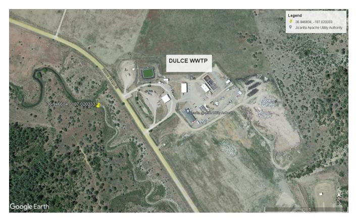
Under the Standard Industrial Classification Code 4952, the applicant currently operates a domestic wastewater treatment facility. The Dulce wastewater treatment plant consists of headworks, two sequencing batch reactors, a flow-through ultraviolet (UV) system and an aerobic digester. Only air is added to the batch reactors. No additional chemicals are added by the facility during treatment. The facility has a design flow capacity of 0.6 MGD and for a total population served of 2,607.
