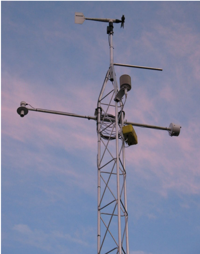
Figure 14. R.M. Young Meteorological System: (from top to bottom) Meteorological Tower with Wind AQ, Directional Cross-Arm, Gill Aspirated Shield for RH Probe, 9-m Aspirated Temperature Sensor Shield and Waterproof RH Circuit Card "Otter" box.
