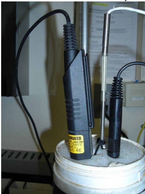
Figure 3. Dostmann probe (left), Eutechnics transfer probe (middle) and Extech probe (right) immersed in stirring bath. More than one temperature transfer device may be certified simultaneously.
