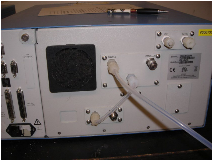
Figure 9. O 3 Transfer Sample Tubing
