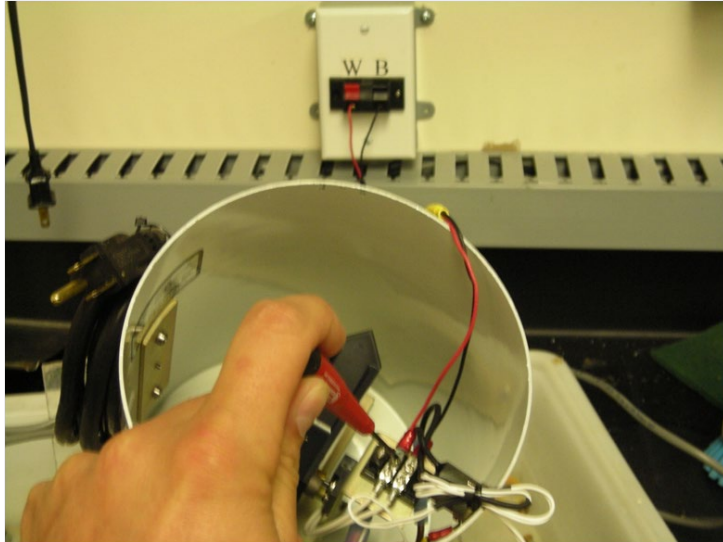
Figure 3. Use wires from wall jack to wire into tipping bucket
