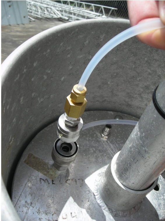
Figure 25b. Flow Transfer Tubing Connected at Flow Calibrator
