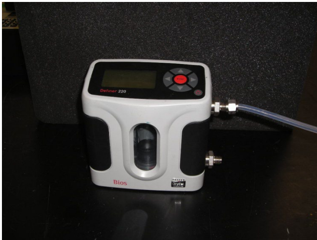
Figure 25b. Flow Transfer Tubing Connected at Flow Calibrator
