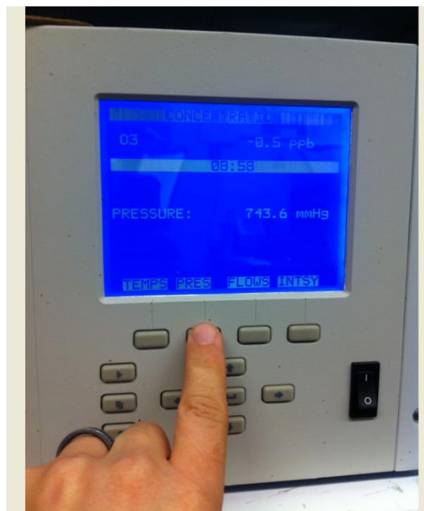
Figure 17. O 3 Analyzer Display of Cell Pressure
