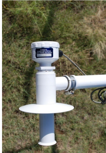
Figure 19. R.M. Young Temperature Probe Installed in Aspirated Shield.
