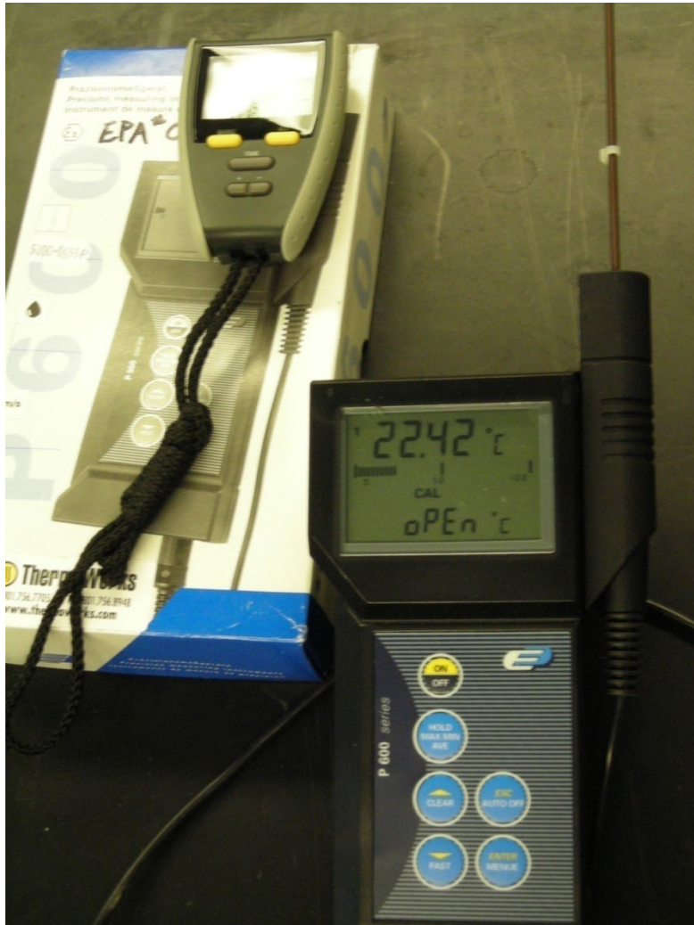
Figure 6. Place digital barometer next to RTD to check temperature accuracy
