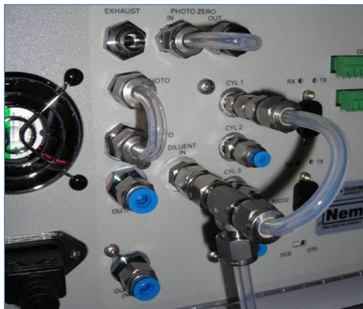
Figure 3. DILUENT IN and CYL1 Connection
