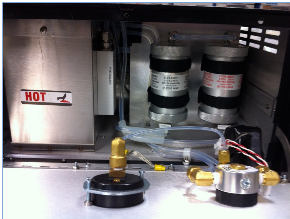
Figure 2. Scrubber Canisters Accessed from Front Panel
