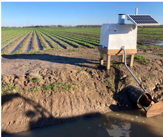
Edge-of-field surface water quality monitoring equipment installed adjacent to a field in Bolivar County, Mississippi, planted with fall cover crops.
