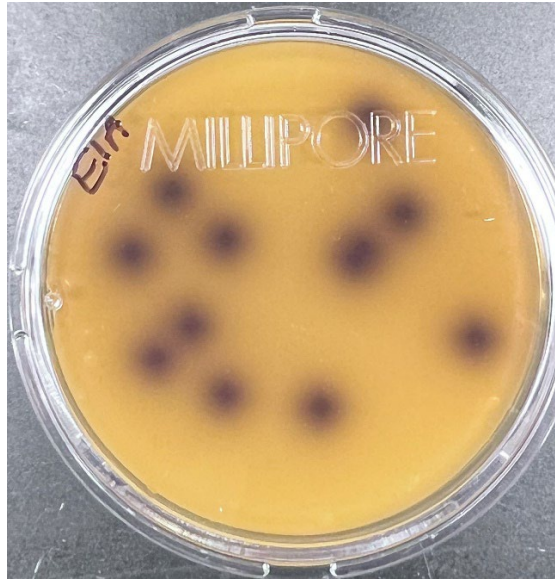
Photo 2. Enterococci colonies are pink to dark red on mE and produce a reddish-brown to black precipitate on the underside of the filter when placed on EIA, while atypical colonies do not produce a precipitate.
