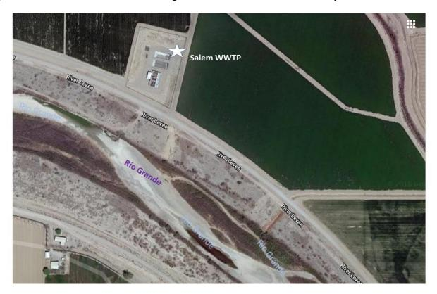
Under the Standard Industrial Classification (SIC) Code 4952, the applicant operates a municipal wastewater treatment plant with a design capacity of 0.20 million gallons per day (MGD) serving a population of approximately 705. The effluent from the treatment plant is discharged into the Rio Grande in Segment 20.6.4.101 of the Rio Grande Basin. The discharge is located at Latitude 32° 41' 36" North, Longitude 107° 12' 30" West.
