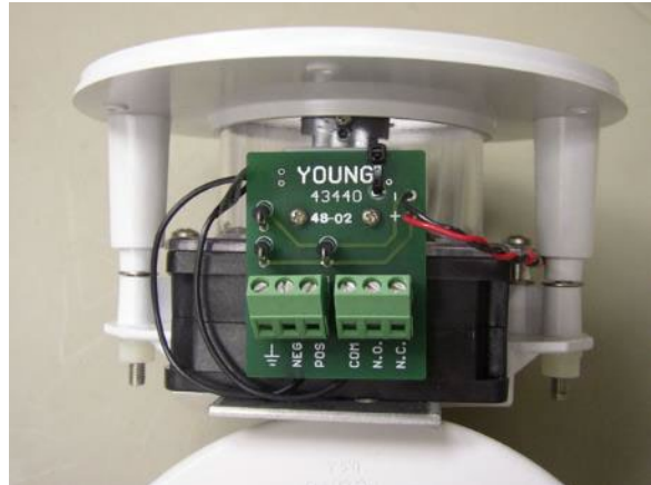
Blower Fan for Aspirated Temperature and Relative Humidity Sensor
