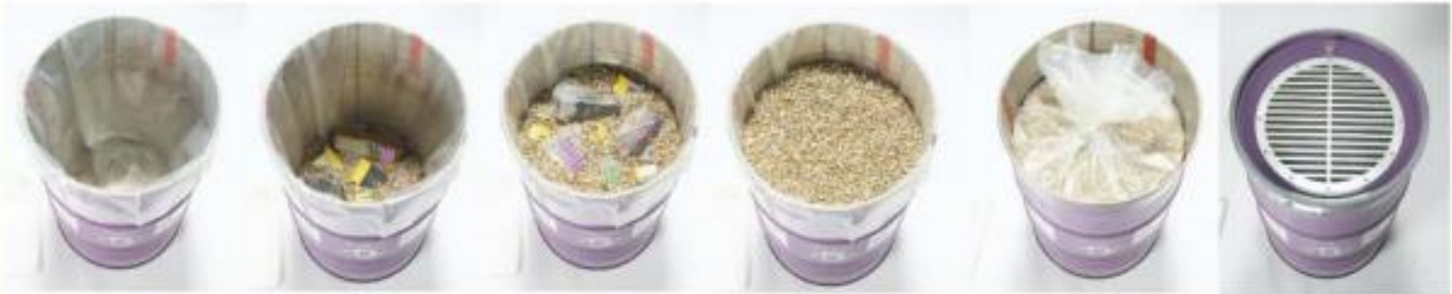
Picture 18. Example of procedure for filling a LIB barrel (Source: INOBAT, LIB barrel)
