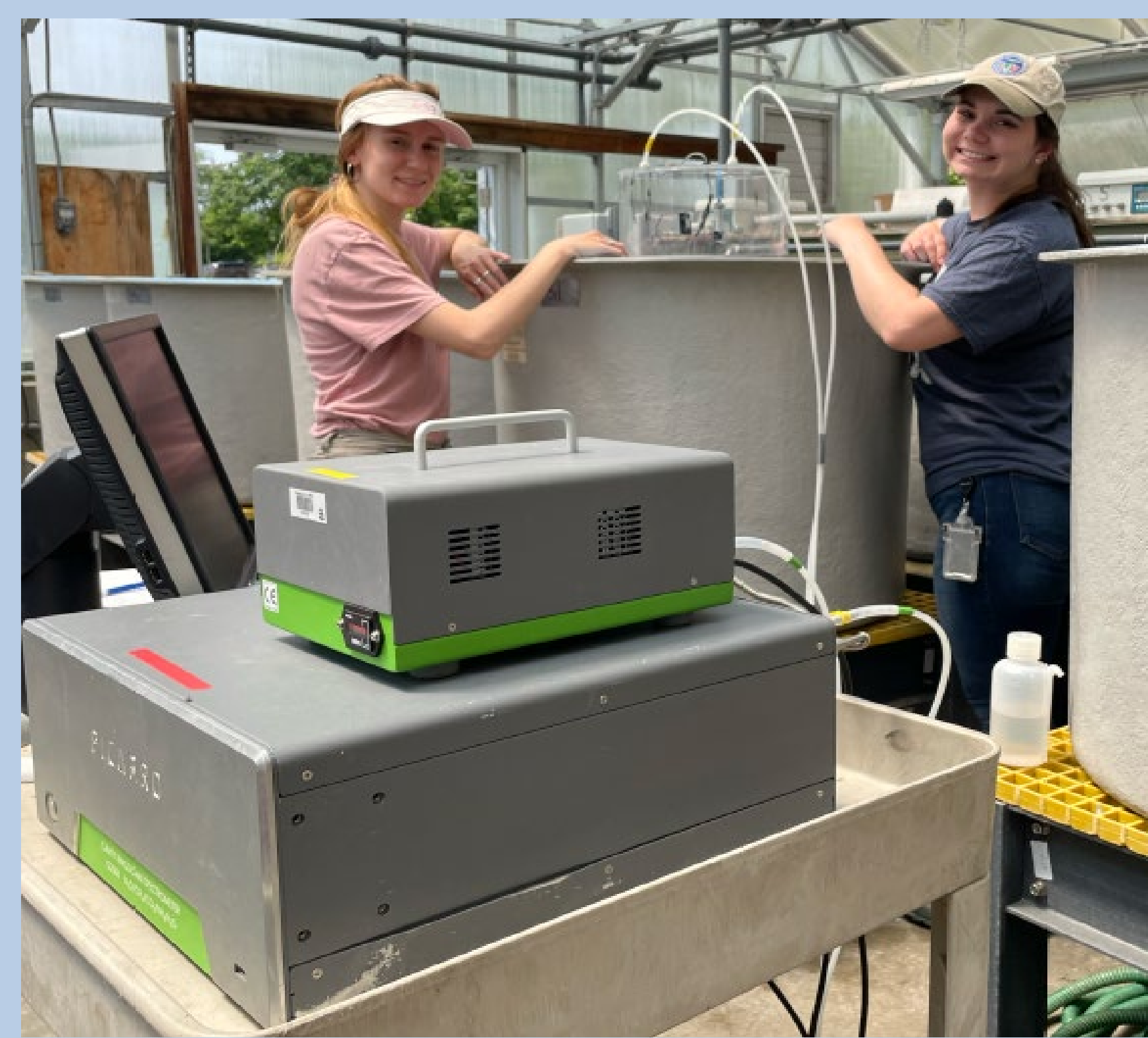
Figure 3. Measuring greenhouse gas fluxes from one of the mesocosms using a floating chamber connected to a Picarro gas analyzer. This instrument simultaneously measures CO 2 , CH 4 , and N 2 O.
