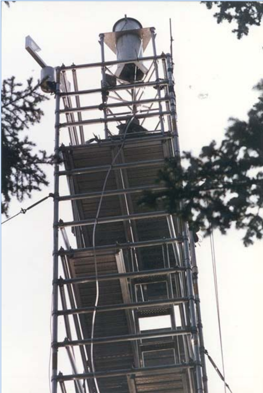
The automated cloud collector (in the down position) on top of the CASTNET tower at Clingmans Dome, TN
