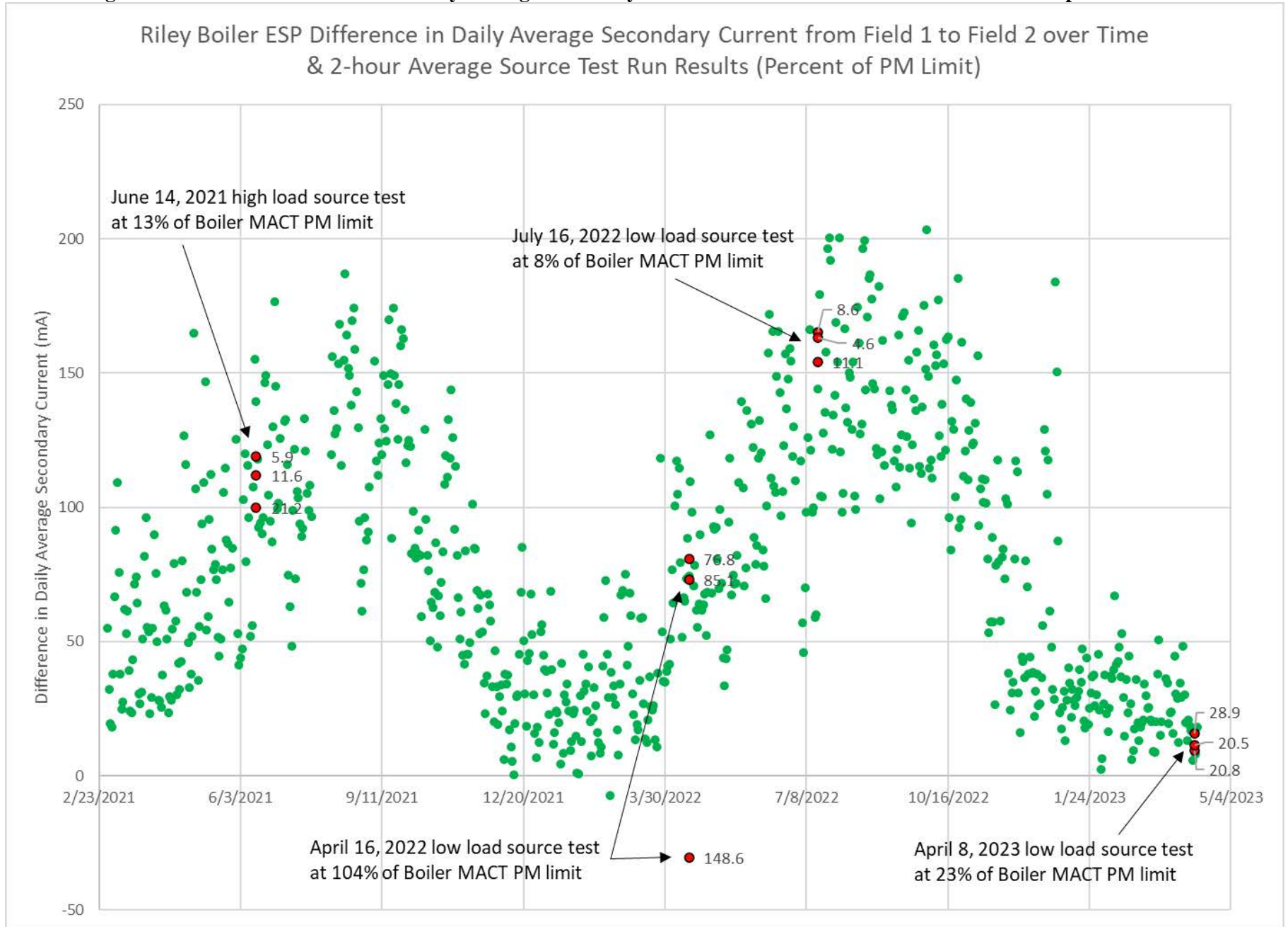
Figure 5-16: PB-2 ESP Difference in Daily Average Secondary Current from Field 1 to Field 2 March 2021 – April 2023
