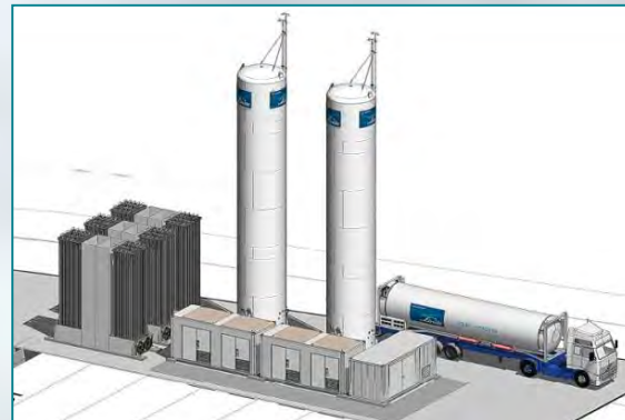
4,300ft 2 footprint for a 75 bus station with 2x 4.5t storage of liquid H 2
