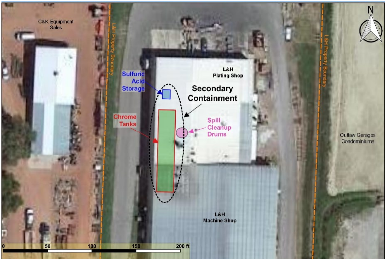
Figure 3 - Chrome Plating Line/Chemical Storage
